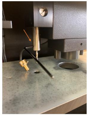
7. Slide sense collar back on to new drill bit and tighten its two set screws
