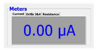
The meters section allows the user to monitor measurements during testing. It allows for monitoring of current, voltage (across drill bits 3&4) and resistance calculated from current and voltage measurements. The measurements are constantly updated in real time.
