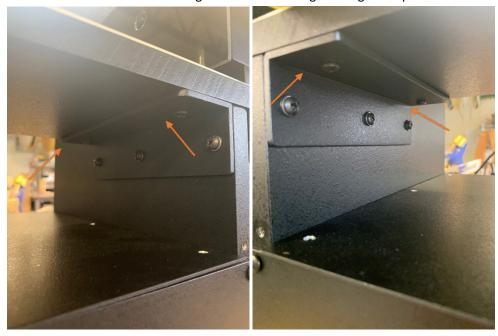
4. The IR receivers are attached to the shelf so cut the wire tie below and unplug them so they can be removed with the shelf.
