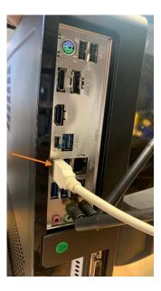
3. Plug the other end of the USB-B cable into the IRT Tester, along with the power cable and air. Power must be 120/220 VAC and air must a minimum of 60 PSI, Clean and water trapped.
